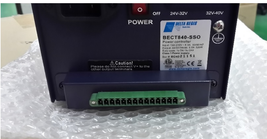
Figure II (new) Transfer semi- assembled with green male terminal connector. Part Number: CA50227A
