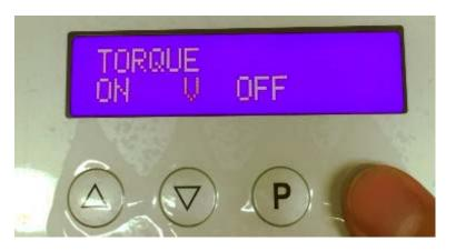
6. The scale "0" will start blinking when enter the torque calibration mode, Click E/C button again to start calibration.
