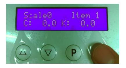
• Please adjust screwdriver torque scale to 0 and start executes calibration, let screwdriver preform the torque test five times on the KTM. (Kilews recommended that set torque auto-zero time to 0.5 second on KTM, which can reduce the time of pressed clear button and shorten the calibration cycle time)
