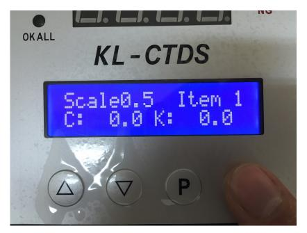
• The calibration software scale will jump to next scale as 0.5 as well, then we can start to test next five times torque value for this scale on KTM.
