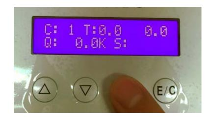
2. keep press up or down button until shows "TORQUE" mode
