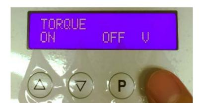
4. Press up button to switch it to "ON" position
