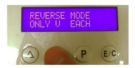
3. When enter to TORQUE mode, click E/C button and tick will start twinkling
